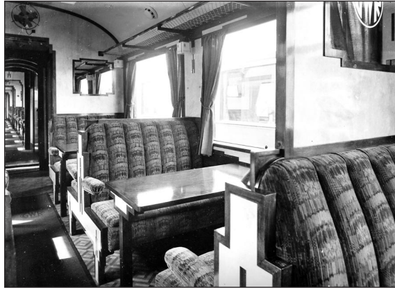
An interior view of one of the first Lots with the Beclawat windows. Dia C68, Lot 1530, No 4568.
